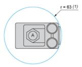
$\emptyset$ A = G 3/8 (1) Minimum clearance zone for screwing-on pressure switch at point A
