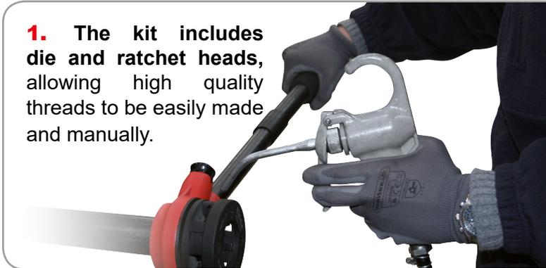
**1.** The kit includes die and ratchet heads, allowing high quality threads to be easily made and manually.
