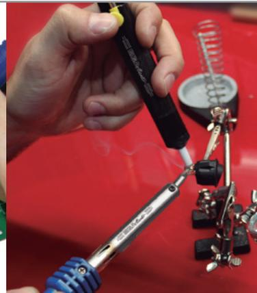
**1.** Thin tip made of copper oxide for high precision works.
