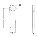
This arm is designed to accommodate a reaction point at a 90 degree angle from the drive.
