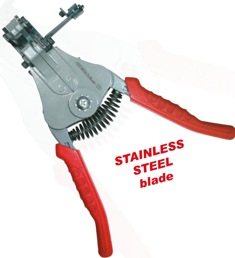
**1.** For the cutting and stripping of insulated cables from 0.5 to 3.2mm diameter and from 0.2 to 8.5mm<sup>2</sup> section in a single step. Just squeezing the handles for opening and closing the jaws will easily remove the isolation from the cable.
