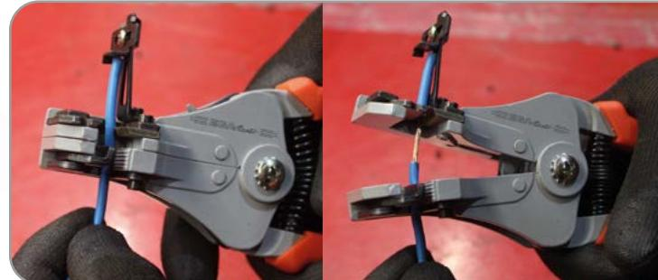
**2.** 3 different models available for cable stripping of different diameters mm/ AWG.
