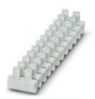
Polypropylene Europe terminal strip, white, for connecting solid conductors and stranded conductors with and without ferrules with a cross section of 1 to 10 mm²
