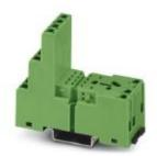
Relay base PR2-B, for industrial relay REL-IR with 2 or 4 PDT, 1/3-level version, screw connections, connection facility for input/interference suppression modules, for mounting on NS 35/7.5
