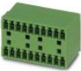
PCB headers, nominal current: 8 A, rated voltage (III/2): 160 V, nominal cross section: 1.5 mm<sup>2</sup>, number of positions: 5, pitch: 3.81 mm, color: green, contact surface: Tin, mounting: Wave soldering, pin layout: Linear pinning, solder pin [P]: 3.5 mm, In combination with MCV plug components, both an MCVW and an MCVR plug must be used.
