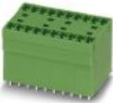
PCB headers, nominal current: 8 A, rated voltage (III/2): 160 V, nominal cross section: 1.5 mm<sup>2</sup>, number of positions: 5, pitch: 3.81 mm, color: green, contact surface: Tin, mounting: Wave soldering, pin layout: Linear pinning, solder pin [P]: 3.4 mm, In combination with MCV plug components, both an MCVW and an MCVR plug must be used.
