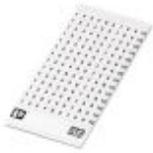
Marker card, Card, white, labeled, horizontal: consecutive numbers 1 ... 10, 11 ... 20, etc. up to 91 ... (99)100, mounting type: adhesive, for terminal block width: 3.81 mm, lettering field size: 3.81 x 2.8 mm
